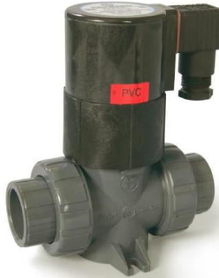
The valves are available in a normally closed design rated at a non-shock 150 PSI at 70 °F . 110V is the standard voltage with additional voltages 12 VAC, 24 VAC, 220 VAC, 12 VDC, 24 VDC available as options.
