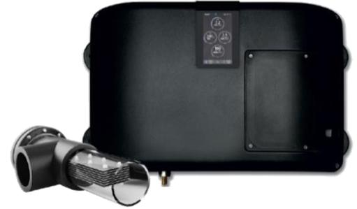
The systems include a control panel made from polymeric materials to prevent corrosion while installed in mechanical rooms. The specially designed housing also provides higher heating dissipation.
