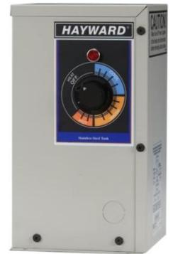
All CSPAXI models have 304 stainless steel tanks for longer life. The electric heating element also has a 304 stainless steel threaded head and a built-in safety sensor to protect the heater against dry firing.
